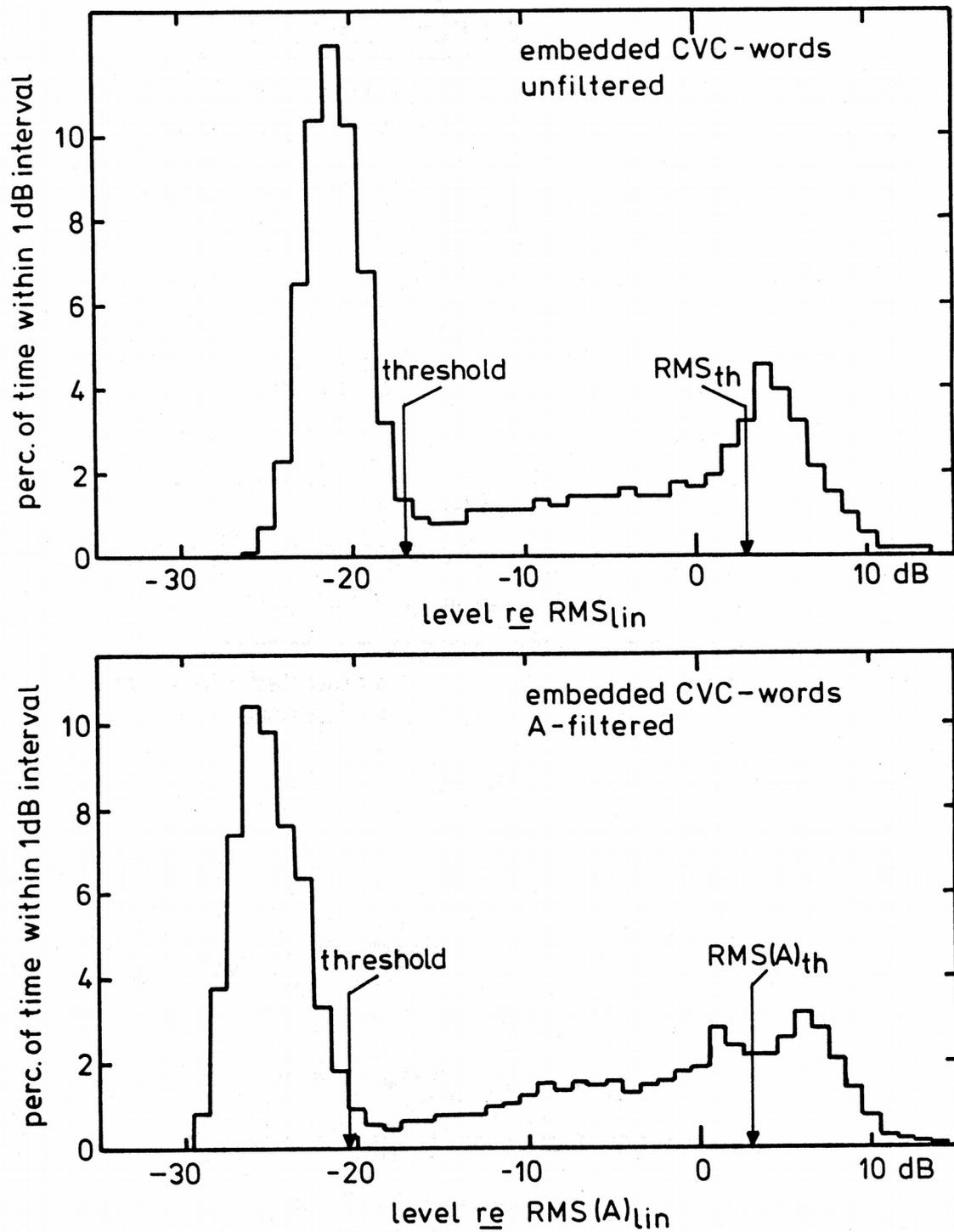
**Fig. 1.** Level distribution histogram of a 150-s speech fragment from embedded CVC-words obtained with envelope sampling after full-wave rectification and integration. The left arrow line represents a threshold value just above the distribution of the background noise during the silent periods.
