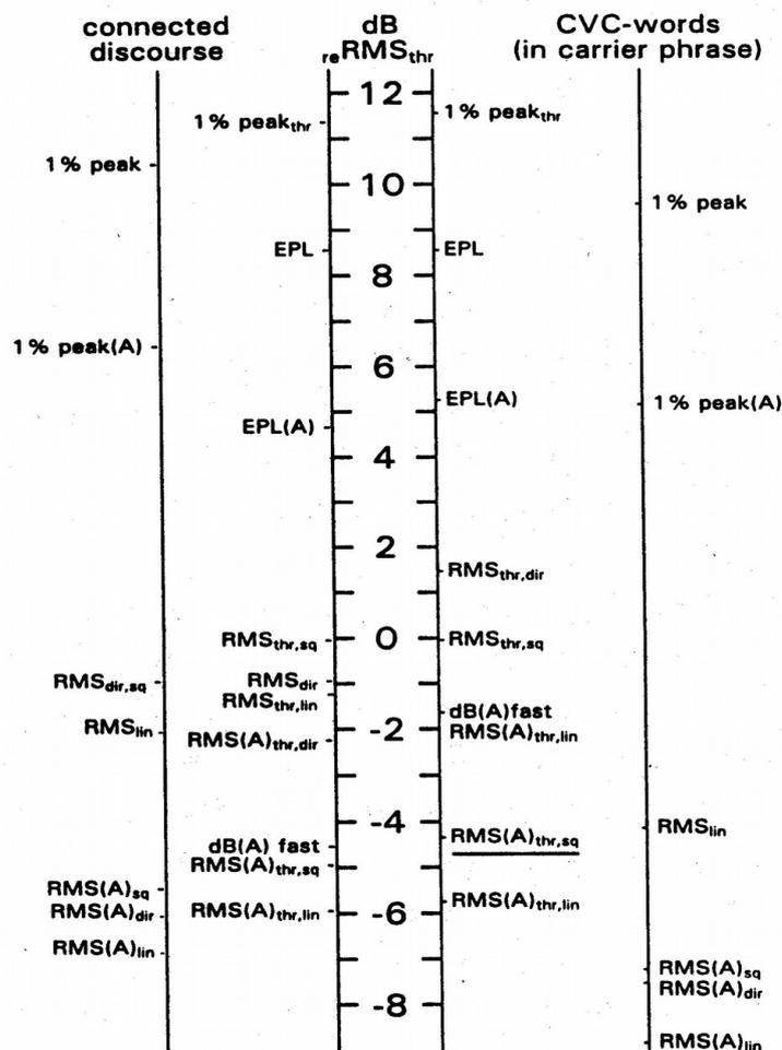
**Fig. 2.** Relative speech levels for different speech-level measures applied to connected discourse and embedded CVC words. The values are relative to the  $RMS_{thr,sq}$  value. For STI measurements (related to CVC-word score prediction) the test-signal level must be adjusted equal to the (underlined)  $RMS(A)_{thr,sq}$  value.
